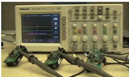
Figure 19: Experimental setup with 3 FireFly nodes
